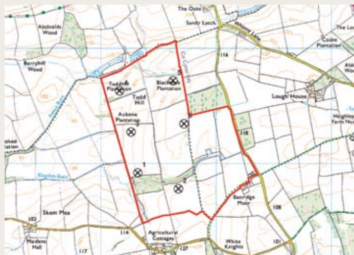
THE INITIAL DESIGN FOR TODD HILL WIND FARM IS FOR UP TO 6 TURBINES, EACH WITH UP TO 2.5 MW CAPACITY
